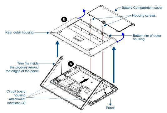
FIG. 5 Removing the MVP enclosure (housing)
